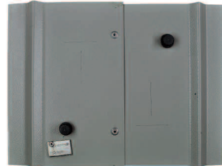
Figure 13. A Colorcoat HPS200 Ultra® test panel after more than 2 years exposure at Brest
