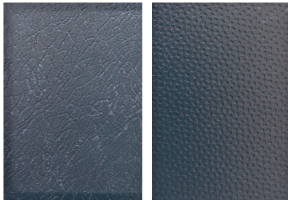
Figure 28. Anthracite standard leathergrain and Colorcoat HPS200 Ultra® after 2000 total hours in UVB test
