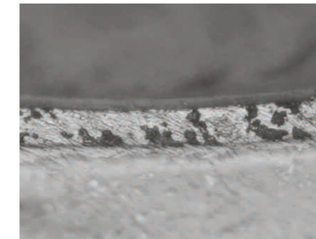
Figure 9. Galvalloy® microstructure after corrosion
