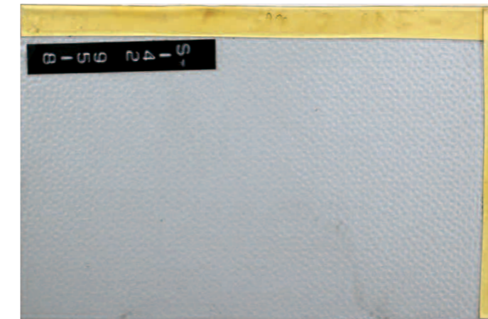
Figure 15. Colorcoat HPS200® with Galvalloy® metallic coating – 10 years exposure at Bohus Malmon, Sweden.
