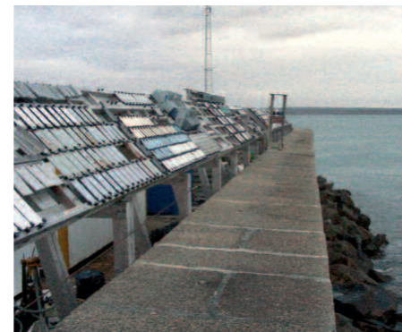
Figure 14. Tata Steel weathering site, Brest C5 marine site
